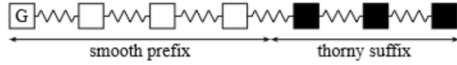
Fig. 9. After the protocol update the adversarial velvet suffix proof consists of an initial part of smooth blocks possibly followed by thorny blocks.
