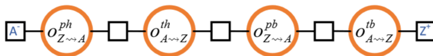
Figure 12. Splitting a Block Transmission into its Constituent Parts: Header ( ph/th ) and Body ( pb/tb ).
